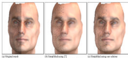
Figure 8: Simplification of a vertex-colored mesh of 130,133 faces down to 1,580 faces.
