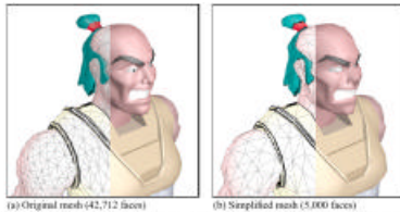
Figure 12: Simplification of a mesh with discontinuities on normal attributes (indicated by the thick lines).
